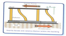
Inertial forces and relative motion within the buildings Source: http://www.iitk.ac.in/nicee/EQTips/EQTip05.pdf
