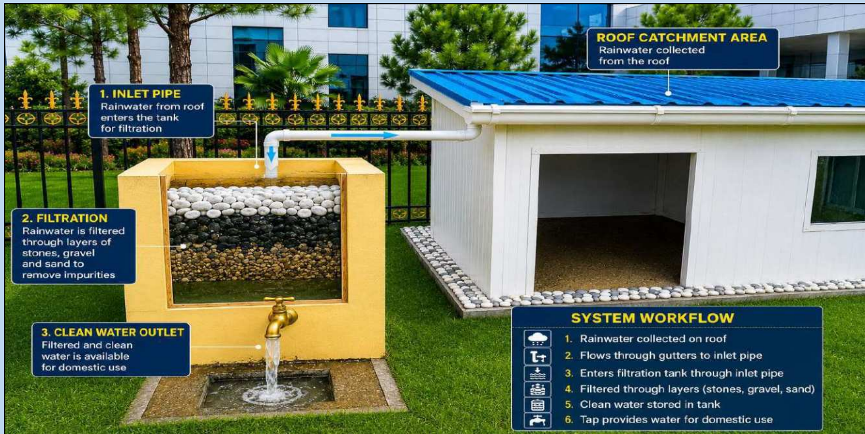
Roof-catchment rainwater harvesting and multi-layer filtration tank, with clean-water outlet tap
