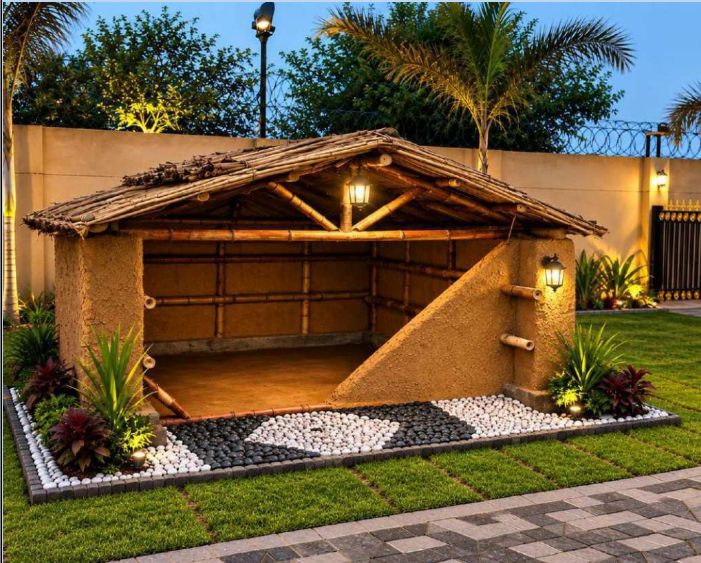
HP2 — Bamboo Frame with Wattle and Daub displayed at NDMA Headquarters, Islamabad
